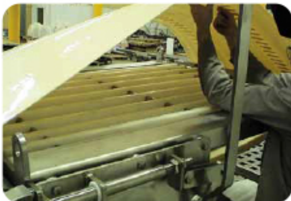
Belt repaired on site.
