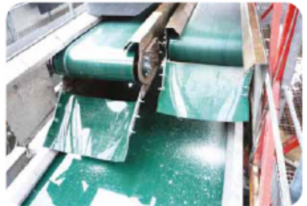
FRPZ-6 with Hammocks : PLASTIC PARTS CONVEYING
