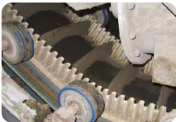
FRG-3 with thermo welded sidewalls and flights: CHEMICAL POWDER (RECYCLED SEWAGE)
